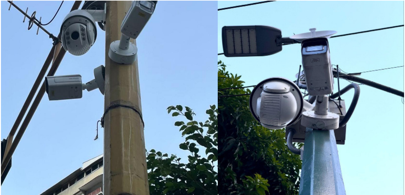
Fixed and PTZ Hikvision cameras in the Altamira sector (left), and the Los Palos Grandes sector (right), Chacao municipality. (Source: VEsinFiltro) 122
