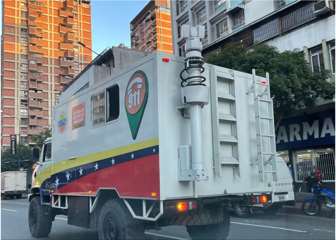
Mobile command unit with CEIEC multi-camera system on a deployable mast. (Source: VEsinFiltro)
